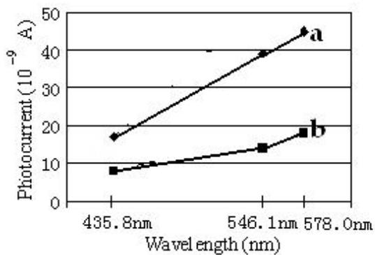
Figure 2 The spectrum energy variation of the converged image with the wavelength when grating combination of 1000L/mm—100L/mm used.
