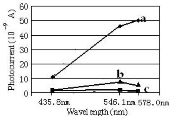
Figure 4 The spectrum energy variation of the converged image with the wavelength when grating combination of 1000L/mm-156L/mm used.
