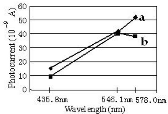
Figure 3 The spectrum energy variation of the converged image with the wavelength when grating combination of 1000L/mm-300L/mm used.
