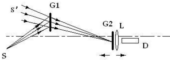
Fig. 1. Optical path of the spectrum imaging and measuring
